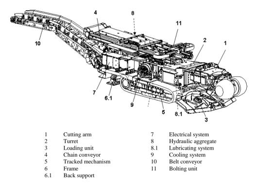
Fig. 3. Scheme of MH-620 Sandvik roadheader (Tkaczuk and Czechowski, 2011)
