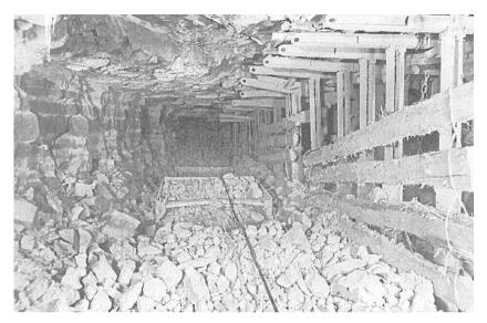
Fig. 1. Hauling of the output from the longwall by the use of a scraper loader (Paździora, 1999)
